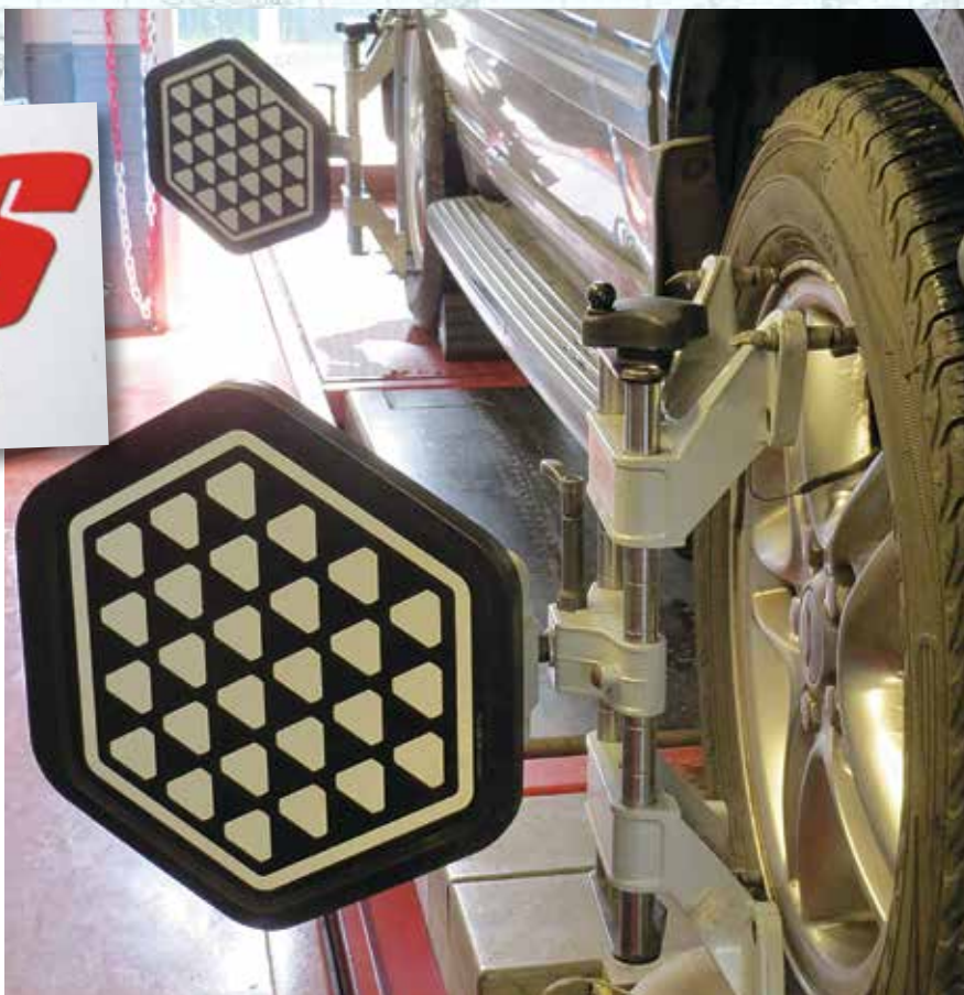
Wheels are fitted with laser alignment hubs
