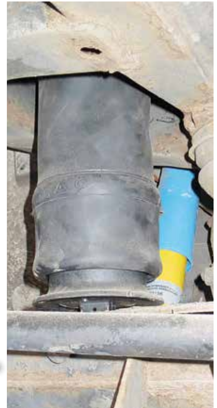
New Britpart air spring in position with Bilstein damper
