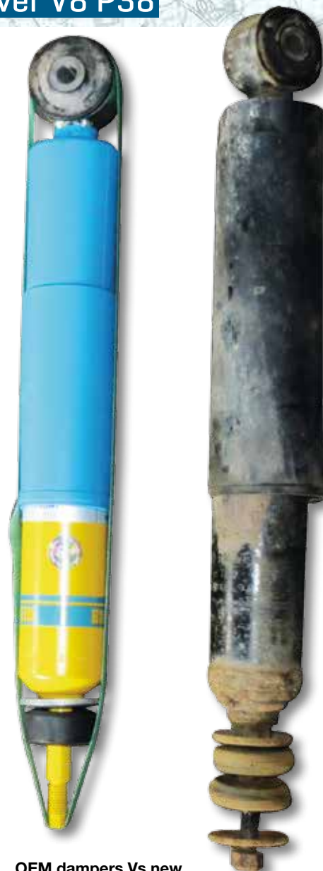
OEM dampers Vs new upgraded Bilstein units: Night & day
